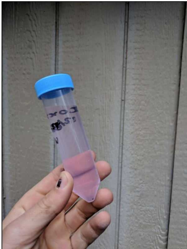
Figure 2. Water sample taken from a domestic Trinity well that showed a positive dye detection. The well is located about 1.25 miles downgradient from the injection site.
