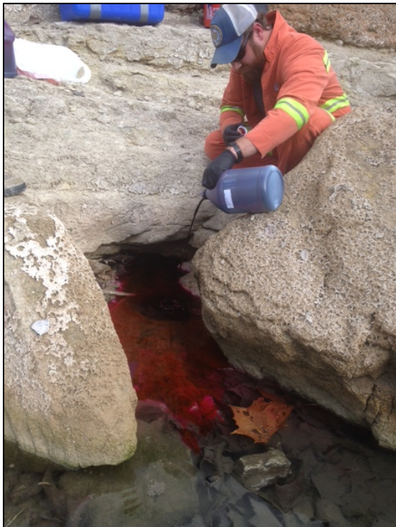
Figure 1. Dye injection into a recharge feature (swallet) within Onion Creek where surface water enters the subsurface through a small opening.
